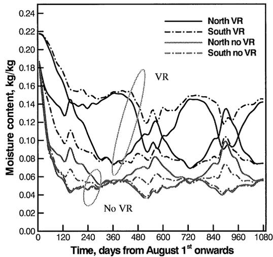
Fig. 7. Moisture contents at three depths of aerated concrete layer for North and South facing walls. Walls without exterior EPS insulation.
