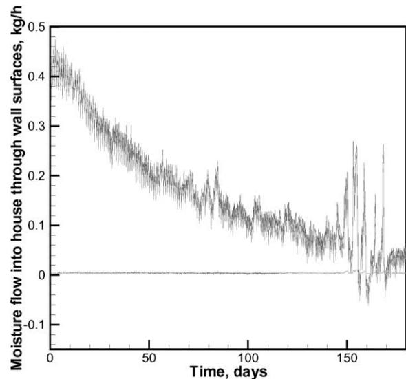
Fig. 13. Moisture flows into the building from the walls. Flat lines are for the vapor retarder cases and the decreasing curves for cases with vapor open interior surfaces.
