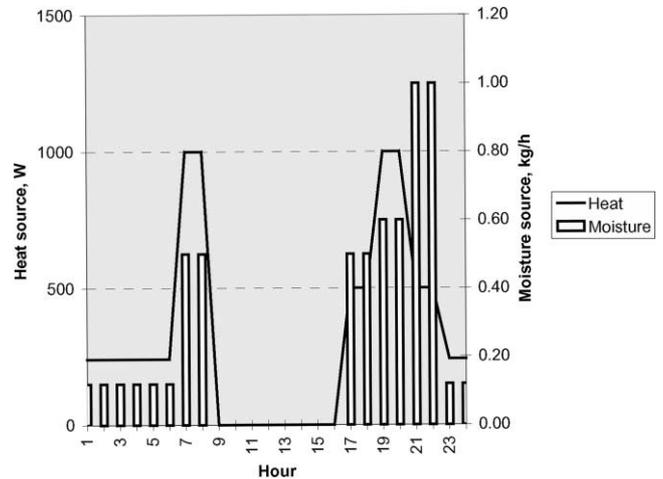
Fig. 2. Heat and moisture sources in the building at various times of day. Daily heat and moisture sources total 7.9 kWh and 6.1 kg.
