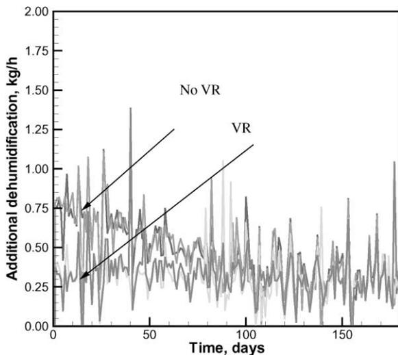
Fig. 12. The difference between the real dehumidification and the dehumidification of outdoor ventilation air to indoor air humidity. For cases with vapor retarding paint the difference is caused by interior moisture sources  $6.1 \text{ kg/day} = 0.25 \text{ kg/h}$  on average.
