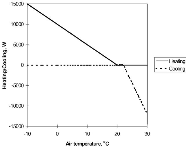
Fig. 3. Maximum heating and cooling as a function of temperature. In x-axis outdoor air temperature for heating and indoor air for cooling. Heating is reduced linearly as indoor temperature rises from 20 to 22°C.
