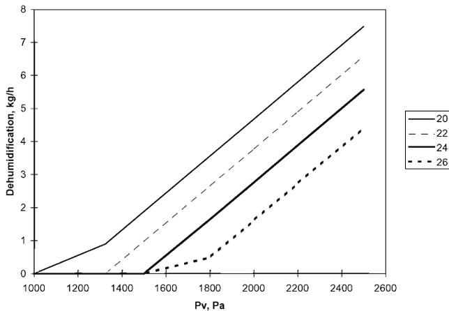
Fig. 4. Dehumidification as a function of interior air vapor pressure (x-axis) and interior air temperature (20–26°C, various curves).
