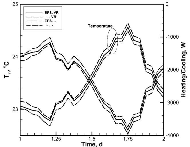
Fig. 10. Indoor air temperature and heating/cooling.
