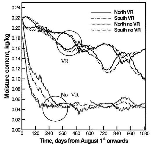
Fig. 5. Moisture contents at three depths of aerated concrete layer for North and South facing walls. Walls with 25 mm exterior EPS insulation.
