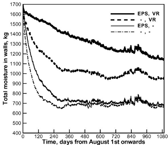
Fig. 8. Total moisture content in the building envelope as a function of time (starting from August 1st).
