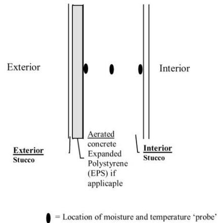
Fig. 6. The graphical layout of the parametric cases (Positioning of numerical moisture and temperature probes).
