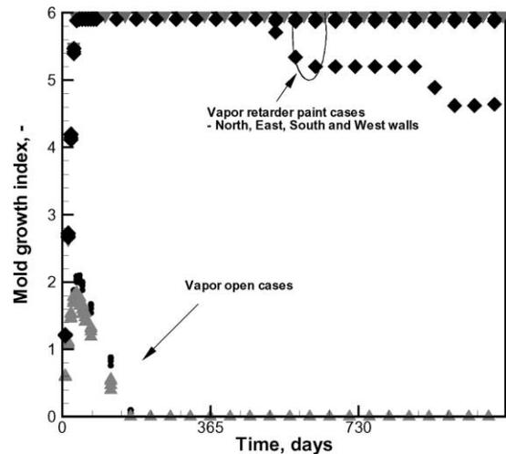
Fig. 14. Mold growth index on the interior surfaces (behind vapor retarder if applicable) of the walls with and without vapor control.
